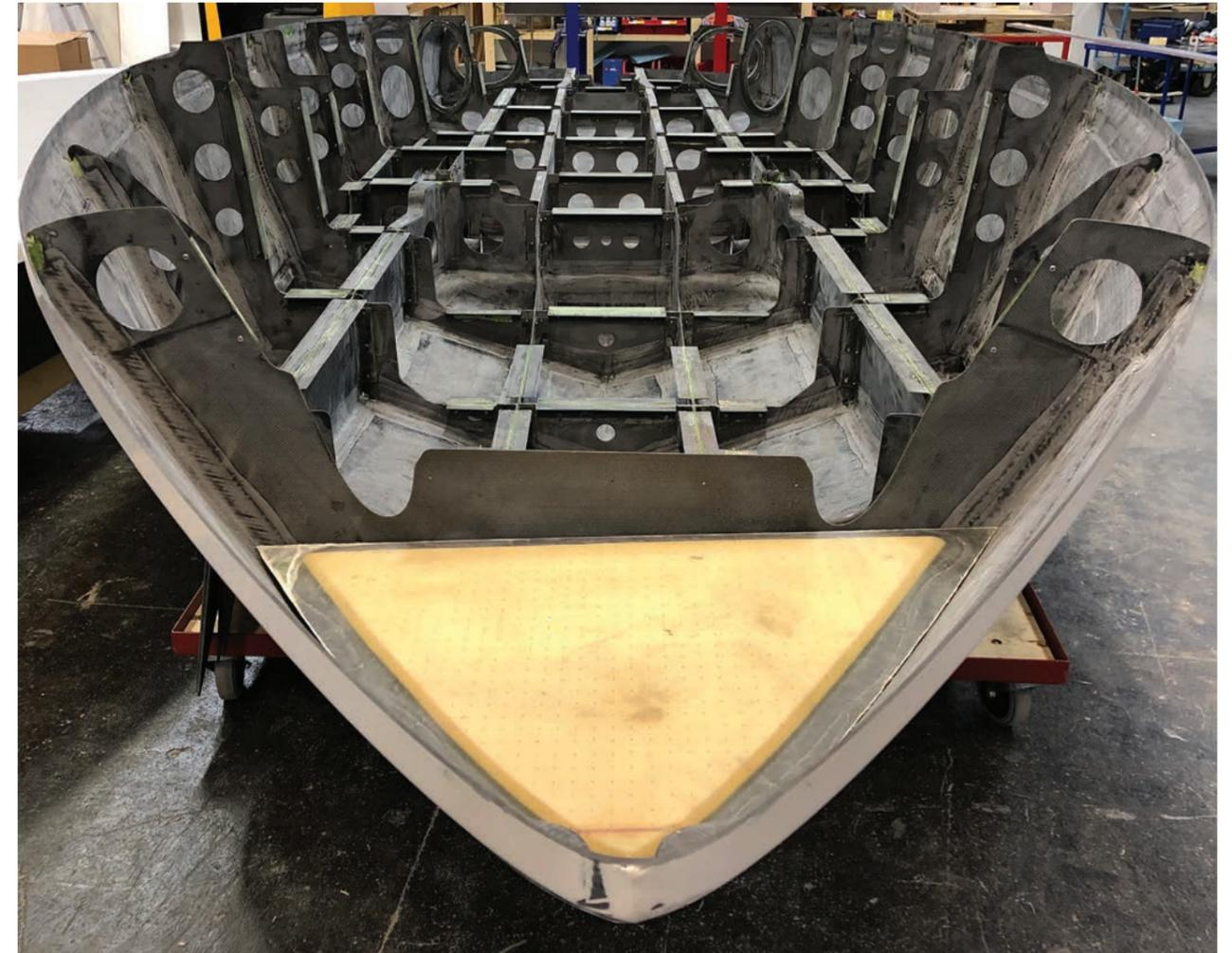
thicknesses below the waterline and only 1.9mm above water, yielding a total weight of only 90kg, and a strong, light deck structure of only 90kg as well... In total, the boat weighs only 1,300kg, about half the weight of other boats in this class.
