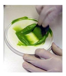
The extra mixing nozzle assures a good mixing between resin and hardener, that is showed by the homogenous green colour at the output.
