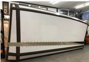
In 2020, Greenboats was commissioned by a wind turbine manufacturer to design and manufacture a sustainable NFC nacelle. The resulting 7.3m long structure has a surface area of approximately 100m2 and was engineered by Greenboats to satisfy all DNV-GL load cases required for an offshore turbine nacelle, including 200km/h max wind loads and 2KN loads on the guard rails.
