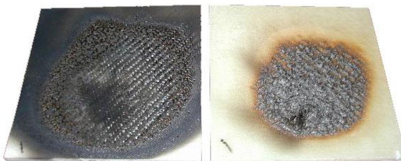
E glass / Epoxy laminates after fire tests: Brominated Epoxy / SR 1126 Epoxy
